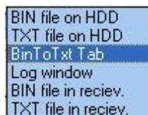
'**Bin file on hdd**' will create the logs in a bin file and save to your hard drive
